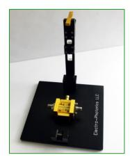
The FRFS-MSA0670-001 is a high performance RF/Microwave production type fixture for testing Avago MSA-0670 cascadable silicon bipolar MMIC amplifier. This fixture is constructed to provide repeatable measurements in production environment. The FRFS-MSA0670-001test fixture features a fast load/unload clamshell type cover.
