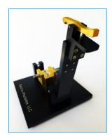
The FRFS-BCR122-001 is a high performance RF/Microwave production type fixture for testing Coilcraft BCR-122 ruggedized conical inductor. This fixture is constructed to provide repeatable measurements in a production environment. The FRFS-BCR122-001 test fixture features a fast load/unload clamshell type cover.
