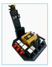
The FRFS-48BGA is a high performance RF/Microwave production type fixture for testing various devices in a 48-pin ball grid array (BGA) package. This fixture is constructed to provide repeatable measurements in production environment. The FRFS-48BGA test fixture features a fast load/unload clamshell type cover with 5 RF and 4 DC ports.
