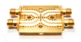
The 722-0006-01-E01 is a high performance RF/MW evaluation board for SMD .250 x .200 couplers. Each board comes with four high performance end launch connectors that are easy to assemble; just slide-on and solder. This board is compatible with many manufacturers' SMD couplers. Save design time and high cost of building a whole panel.
